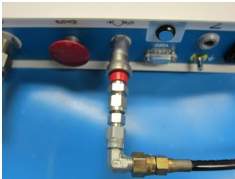
Figure 4: N<sub>2</sub>O Inlet Connection
