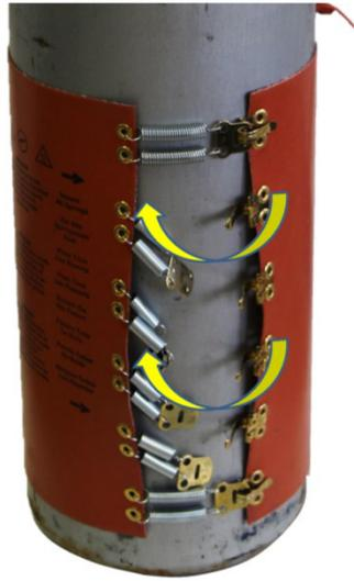
Figure 8: Secure All Tensioning Spring Retainers
