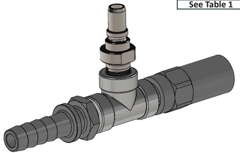
*Figure 25: Exhaust Hose Connector Assembly – A001150*
