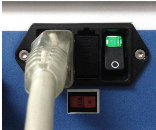
Figure 10: Turn-On AtriCure cryoICE BOX with Switch
