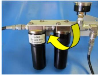
*Figure 23: Filter Housing Removal*
